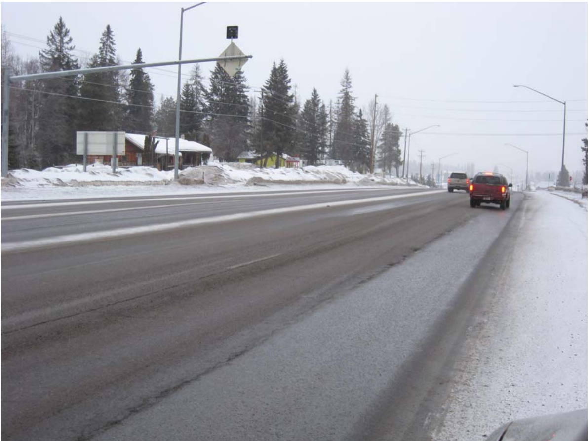
Figure 3 Ice Slicer in the near lane, white salt in the far lane. Notice the consistent ribbon effect in the near lane.
