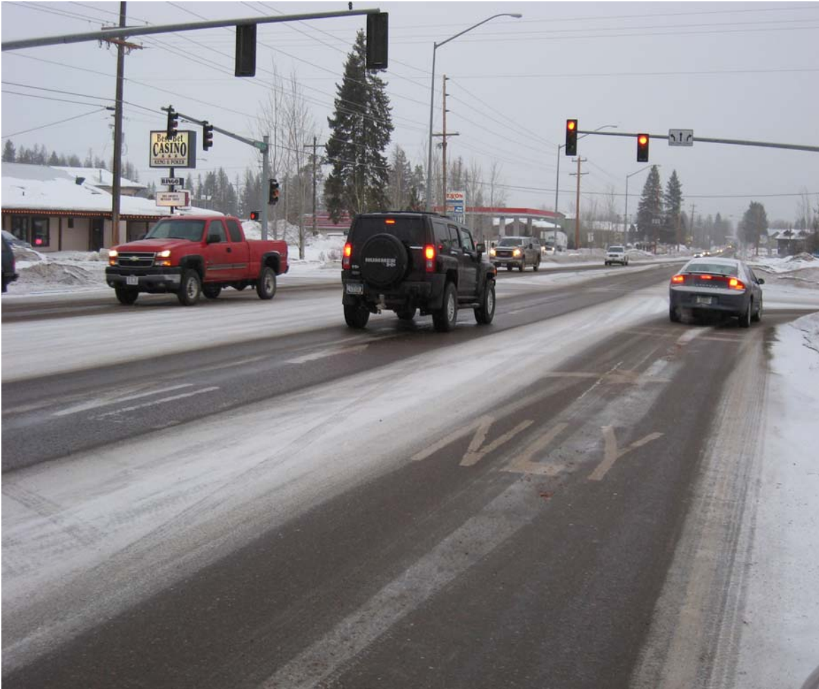
Figure 2 Ice Slicer in the near lane, white salt in the far lane
